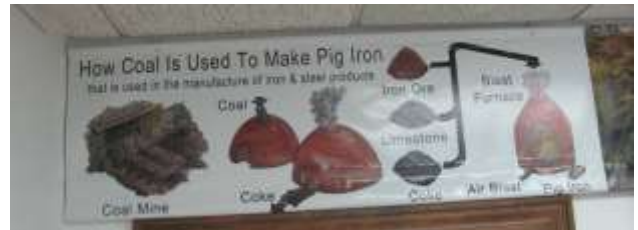
This chart explains how coal was turned into coke in the process of making Pig Iron.
